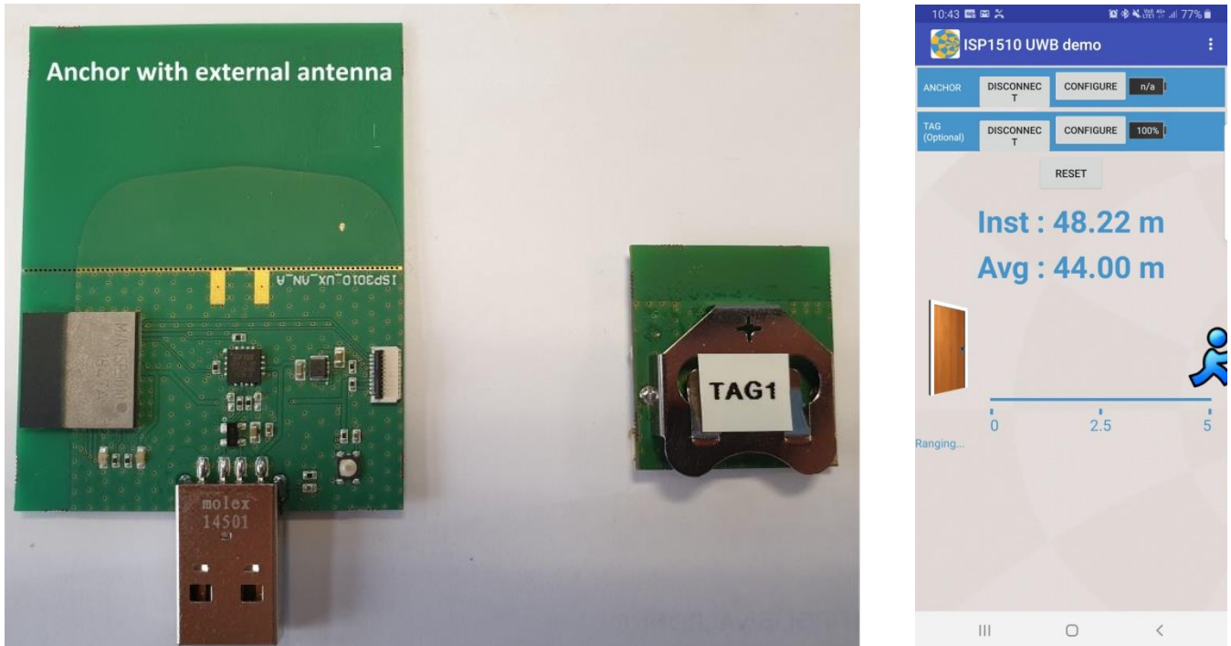
Figure 6: ANCHOR ISP3010 with external antenna VS TAG ISP3010 with LIPO battery
