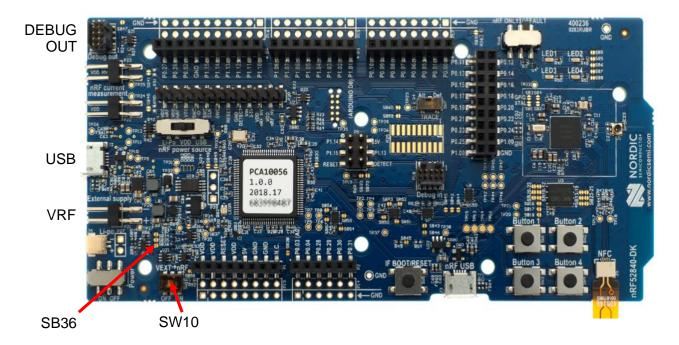
SB36 should be short circuited with a solder bead so that power from the USB and associated regulator is connected to the External supply P21 as an OUTPUT.
