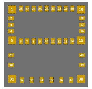
ISP1302 pad placement and pin assignment for the LGA QFN package
