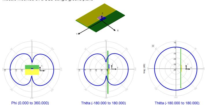
Gain measurement in dBi @ 2.45 GHz
