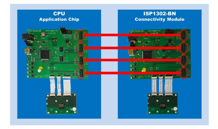
For SPI interface, connect all the following pins on the highlighted connectors:
