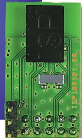
Insight SiP ISP091201 module is based on Nordic's proven µBlue reference design
