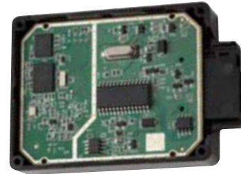
1. M/A-COM Technology Solutions' GPS module includes a GPS antenna, GPS receiver, microprocessor, memory, CANbus transceiver,
