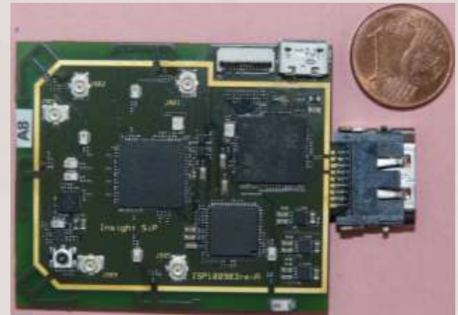
WHDI RECEIVER MODULE - ISP100903 - 47 x 41 x 4.5MM
